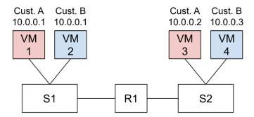
Assume the packets in the underlay network look like the one below. The virtual network header has one field, the ID, which has the name of the customer in it.
