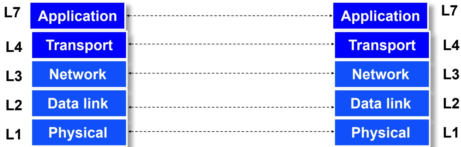
Communication between peer layers on different systems is defined by **protocols**
